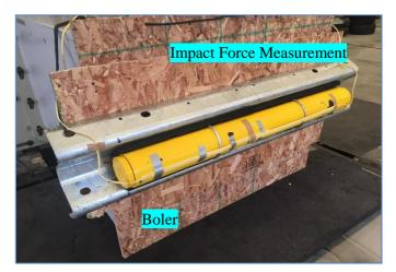
Figure 6 : The specimen was mounted on the rigid offset barrier block
