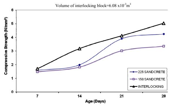
Figure 2: Compressive Strength of Sandcrete and Laterite Interlocking Blocks
