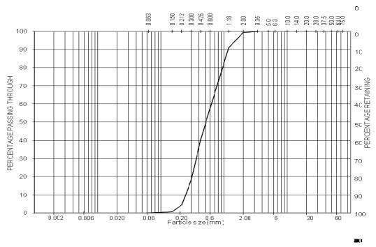
Figure 1: Grading curve for fine aggregates used
