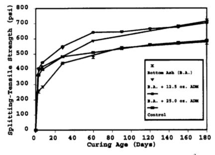
**Figure 5:** Splitting – tensile strength of concrete containing 600lb/yd<sup>3</sup> (365kg/m<sup>3</sup>) cement Source: Ghafoori & Bucholc, 1996
