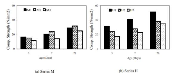
Figure 4: Compressive strength for M & H series Source: Bai, Ibrahim & Basheer, 2010
