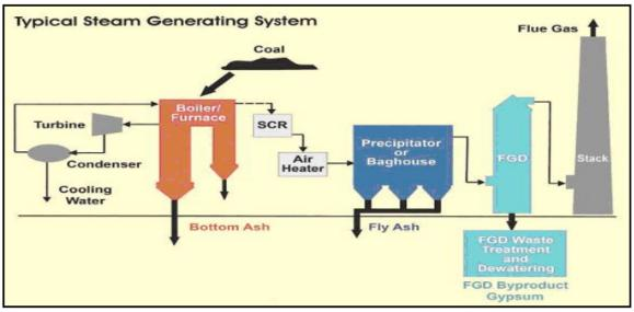
Figure 1: Typical thermal power plant & resulting waste generated Source: NETL, 2006
