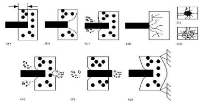
Figure 1. Explains the local impact phenomena caused by hard projectile. (a) Penetration,(b) Cone cracking and Plugging, (c) Spalling, (d) Radial cracking (i) front face and (ii) back face, (e) Scabbing, (f) Perforation, and (g) Global phenomena.
