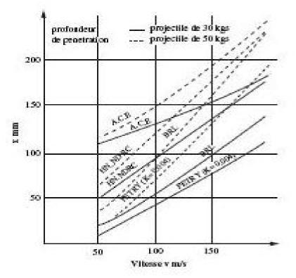
Figure 4. Shows the comparison of various empirical formulae for penetration depth (x), [21].
