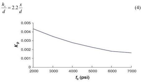
Figure. 2. Variation of concrete penetrability  $K_p$  with the unconfined compressive strength of concrete ( $f_c$ ).
