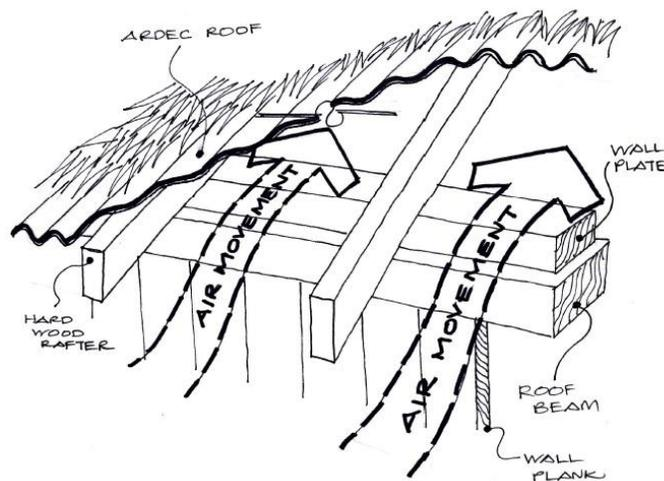
**Figure 10:** Gaps between rafters and roofing that may allow air movement
