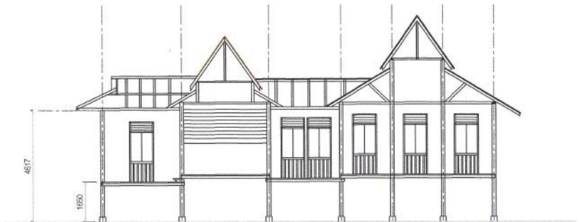
**Figure 6:** Cross Section of Sri Banai House
