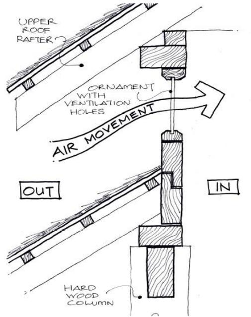
**Figure 14:** Air Movement Flow between Roofs
