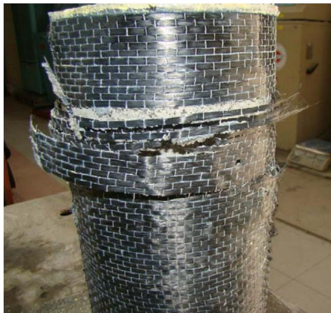
**Figure 3:** CFRP rupture after compressive test
