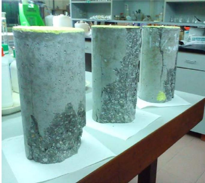
Figure 4. Pre-defected concrete specimens
