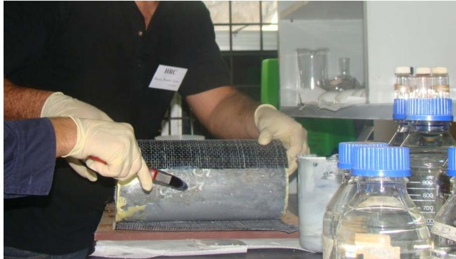
**Figure 2:** Fully wrapping of CFRP to repair pre-damaged concrete specimen
