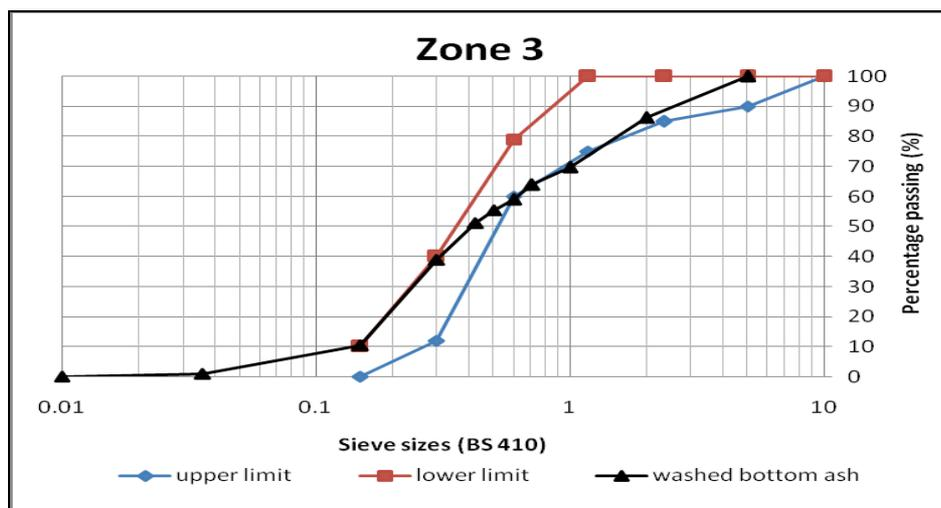
Figure 4: Grading curve of bottom ash for Zone 3
