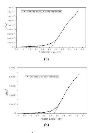
**Fig. 3**  $(\alpha h \vartheta)^2$  versus photon energy of CdO thin film (a) before and (b) after irradiated by laser.
