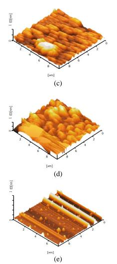
Fig. 1 3-Dimensional AFM images of NiO-YSZ thin film annealing at 600 °C with different layer (a) 1 layer, (b) 2 layer (c) 3layer, (d) 4 layer and (e) 5 layer.
