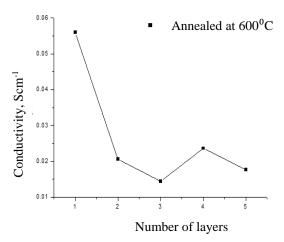
Fig. 2 the graph of conductivity versus number of layers.
