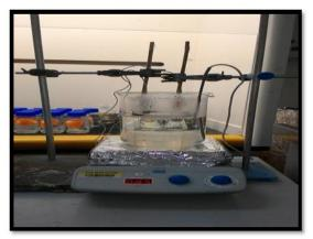
Fig. 1 ZnO electrodeposition apparatus setup
