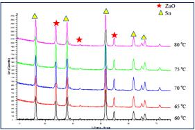
Fig. 2 XRD pattern of  $2\theta$  for each sample with different temperature of water bath.
