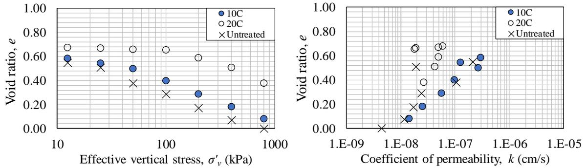
**Fig. 4** Compressibility (left) and permeability (right) graphs of cement-admixed DMS sample.
