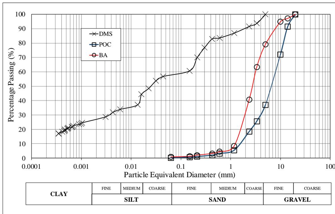
**Fig. 3** Particle size distribution of the materials used
