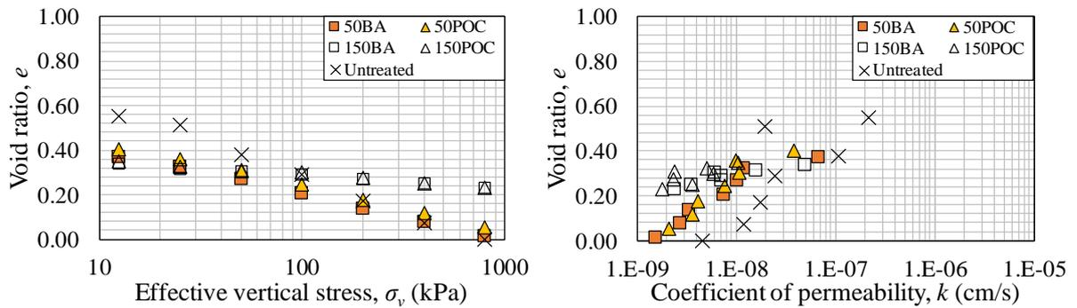
**Fig. 5** Compressibility (left) and permeability (right) graphs of WGM-admixed DMS sample.
