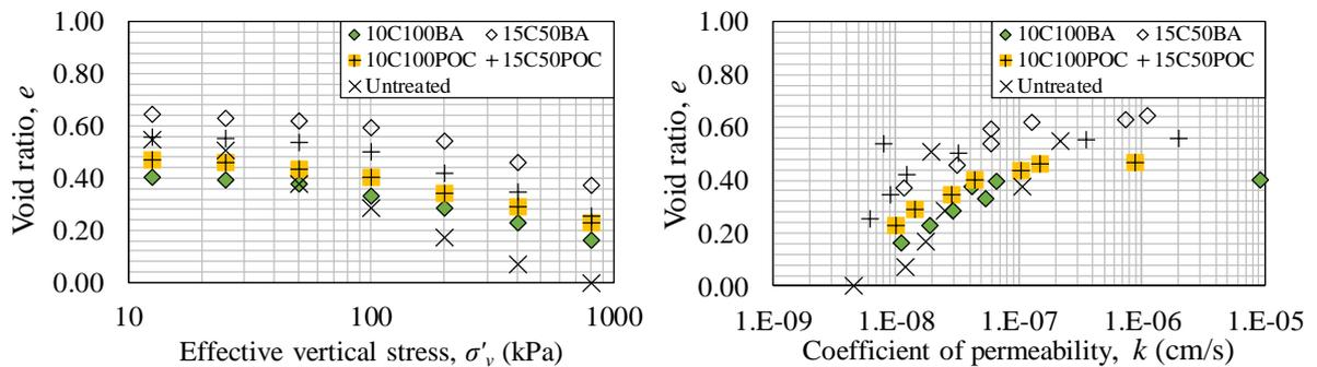
**Fig. 6** Compressibility (left) and permeability (right) graphs of cement-WGM-admixed DMS sample.
