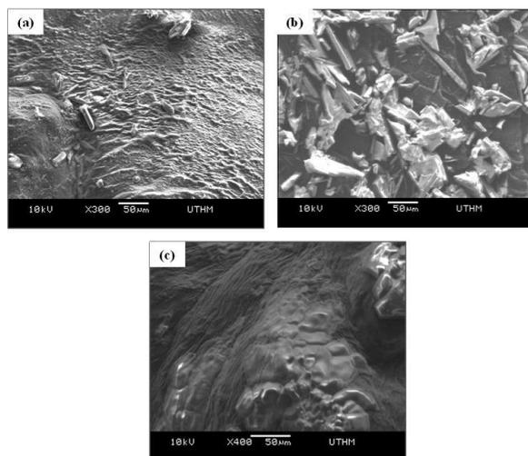
**Fig. 1** SEM image of (a) PVA hydrogel, (b) PVA/6%Chitosan hydrogel and (c) chitosan hydrogel.
