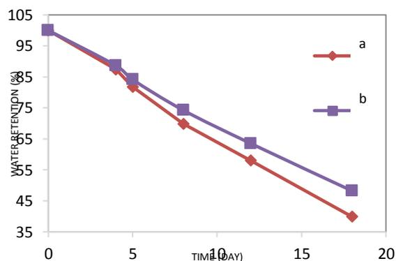
**Fig. 2** Water retention of soil with SAP fertilizer hydrogel. (a) water + dry soil without SAP; (b) water + dry soil + SAP sample A.
