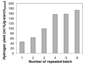
Figure 3: Hydrogen production at different batch cultivations with 10 g/l initial gelatinized dry sago starch concentration using enriched PGK culture at 60 °C
