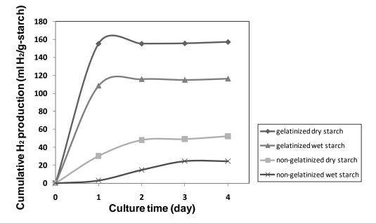
Figure 2: Hydrogen production from sago starch using PGK culture at different starch type with 10 g/l initial starch concentration for 4 days cultivation
