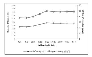
Fig. 2 The optimum ratio of Feldspar-Zeolite for  $NH_3$ -N removal at pH 7 and 200 rpm shaking speed
