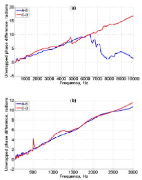
Figure 3: Graph of unwrapped phase difference for (a) smaller container filled with clay at 32 % water content and (b) larger container at 40 % water content.
