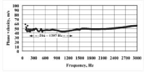
Figure 5: Graph showing variation of phase velocities across the frequencies from the test conducted on the larger container filled with clay at 40 % water content.
