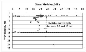
Figure 6: Shear modulus versus wavelength for measurements conducted on the smaller container filled with Oxford Clay at 32 % water content.
