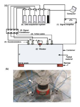
Figure 2: (a) Illustration of the laboratory-scale model and equipment set-up, and (b) photo of the Oxford Clay with sensing accelerometers where the seismic source was located at the centre of the array.
