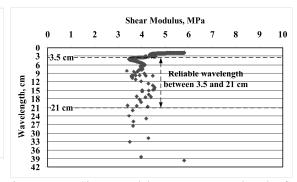
Figure 7: Shear modulus versus wavelength for measurements conducted on the larger container filled with Oxford Clay at 40 % water content.
