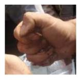
Fig. 8 Von Post Squeezing Test for Pontian Peat Soil
