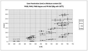
Fig. 15 Graph Water Content (%) with Penetration Depth (mm) of Pontian Peat
