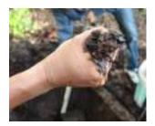
Fig. 6.Von Post Squeezing Test
