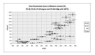
Fig. 14 Graph Water Content (%) with Penetration Depth (mm) of Parit Nipah Peat
