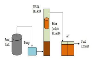
Fig. 1 Design for UASB-AF (R1) and HUASB-AF (R2) treatment system
