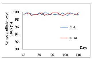
Fig.11 Removal Efficiency of O&G for R2 system
