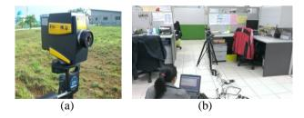
Fig. 4 (a) Laser Doppler Vibrometer (LDV 100), and (b) Measurement at site.
