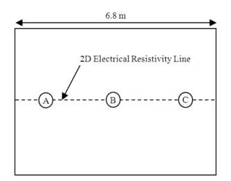
Fig. 2 Schematic diagram (Plan view) of the position of soil sampling and resistivity line alignment.
