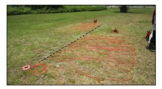
Fig. 1 2D resistivity data acquisition in progress.
