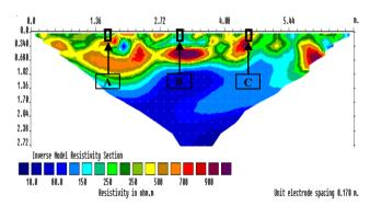
Fig. 3 2D electrical resistivity section and localize extracted ERV (A, B and C) used for further detail study.
