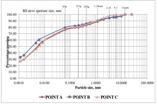
Fig. 4 PSD curve for soil sample at point A, B and C.
