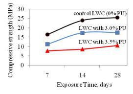
Fig. 4 Effect of varying PU addition in the lightweight concrete on the compressive strength
