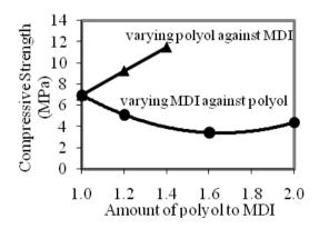
Fig. 3 The effect of PKO-p to MDI ratio on the compressive strength of rigid PU.
