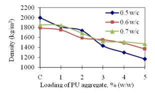
Fig. 2 The effects of palm-based PU addition on the lightweight concrete density with various w/c ratios of the concrete mix.
