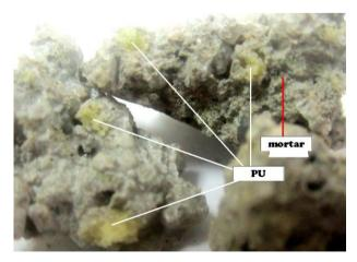
Fig. 5 Polyurethane (PU) covered by cement paste in the broken fragment of concrete.
