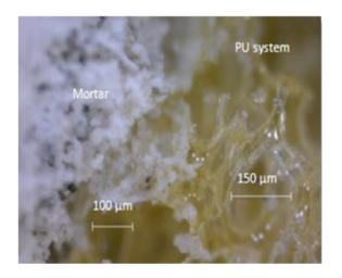
Fig. 6 Interfacial zones between concrete and PU observed using optical microscope at  $500 \times$  magnifications.
