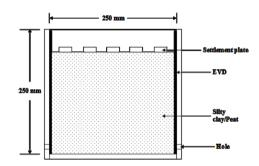
Fig. 6 Test tank with drainage at the bottom of the test bed.
