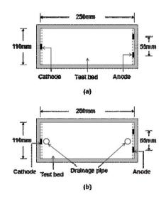
Fig. 7 Plan of test tank showing the 2anodes-1cathode configuration: (a) Drainage at bottom of test bed (b)Drainage through drainage pipe [10].
