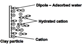
Fig. 2 Clay particle-pore water system.
