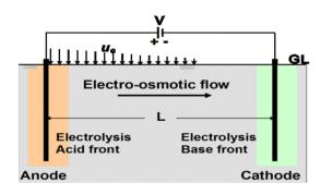
Fig. 1 Electroosmosis and electrolysis reactions [1].
