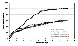
Fig. 9 Influence of polarity reversal on the volume of water drained from Sibu organic soil test beds [1].
