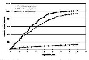
Fig. 8 Influence of pumping interval on the volume of water drained from Sibu organic soil test beds.
