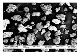
Fig. 5 Scanning electron micrograph of Sibu organic soil [1,10].
