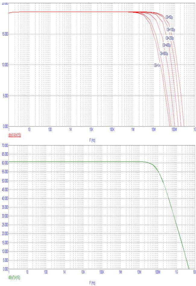
Fig. 12 Frequency response composite transimpedance amplifier
