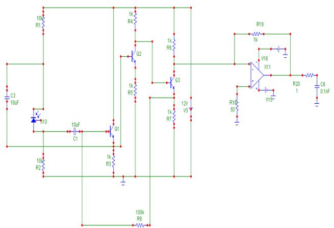
Fig. 11 Composite transimpedance amplifier
