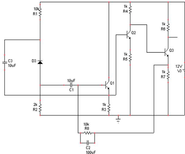
Fig. 6 Bootstrapped transimpedance amplifier circuit
