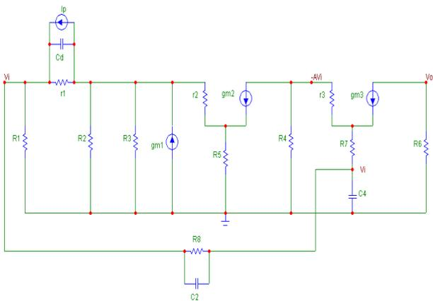
Fig.10 Model hybrid-pi of bootstrapped with capacitor peaking transimpedance amplifier circuit
