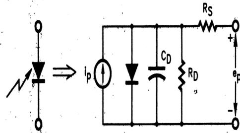
Fig.2 Photodiode circuit model
