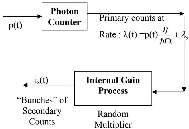
Fig.3 Model of  $i_s(t)$  generation process
