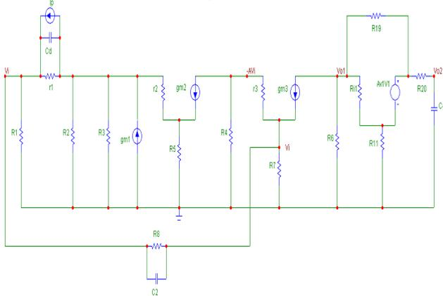
Fig. 13 Model hybrid-pi of composite transimpedance amplifier
