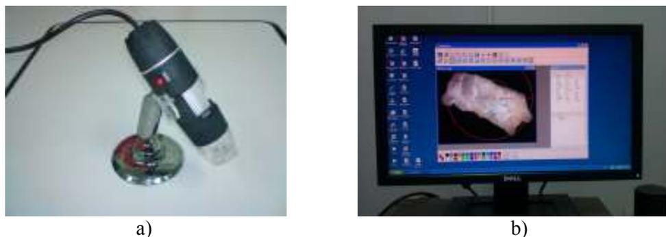
Figure 4: a) Digital microscope used for analyzing particle shapes, b) Digital microscope software.
