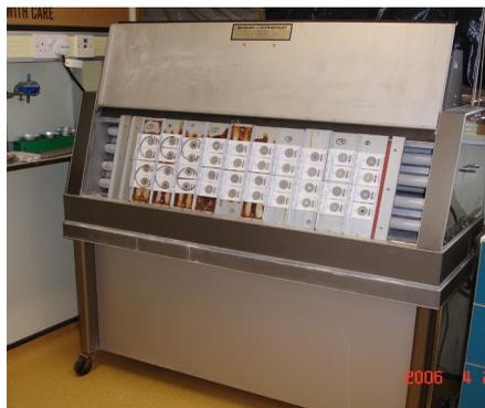
Figure 2.2.3: Q-Panel, accelerated Weatherometer mounted with film samples.
