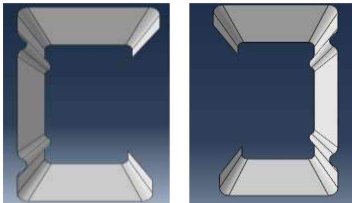
Fig. 1 - C-Sections modeled in Abaqus Software
