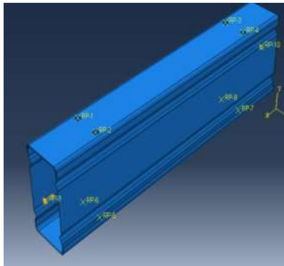
**Fig. 5 - Application of concentrated load at RP 9 (Upper end)**
