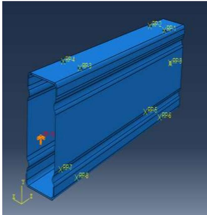
**Fig. 4 - Fixed boundary condition at RP 10 (Lower end)**
