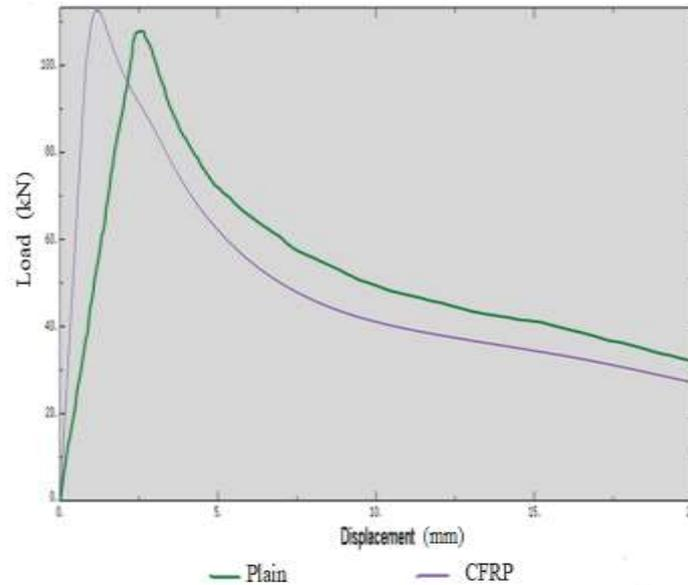
Fig. 9 - Load-lateral displacement of column
