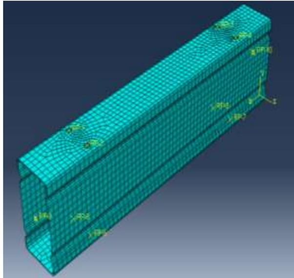
**Fig. 6 - Meshing of a built-up box section**
