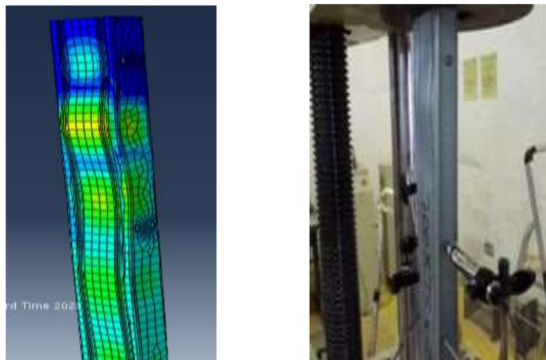
**Fig. 8 - Local buckling from numerical and experimental results**
