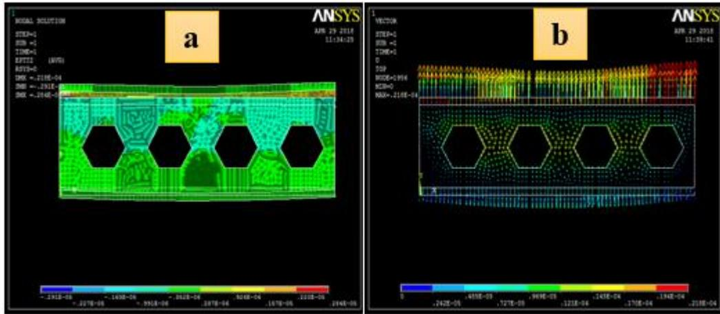
**Fig. 9 - (a) Z-Component total mechanical strain contour plot; (b) predefined vector plot of the section**
