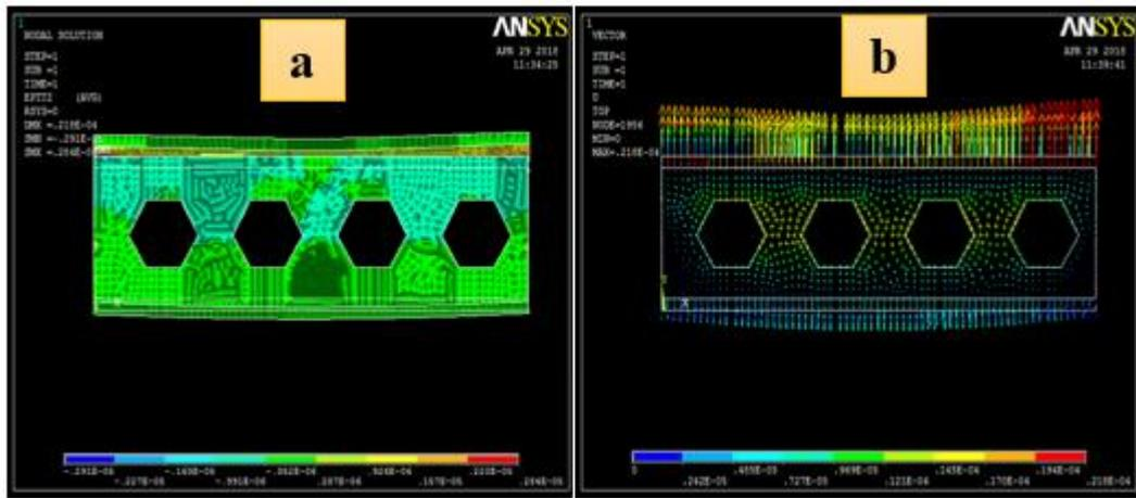
**Fig. 9 - (a) Z-Component total mechanical strain contour plot; (b) predefined vector plot of the section**
