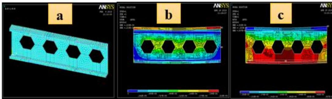
Fig. 7 - (a) Three dimensional area model view in ANSYS window; (b) displacement vector contour plot; (c) X-component degree of freedom solution
