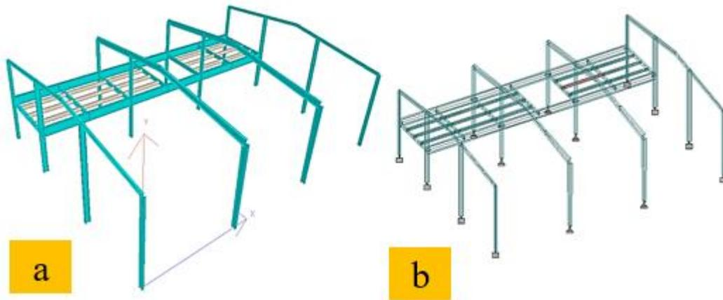
**Fig. 4 - (a) Typical pre-engineered building system STAAD model; (b) dimensions & geometric properties of a hot rolled steel sections**
