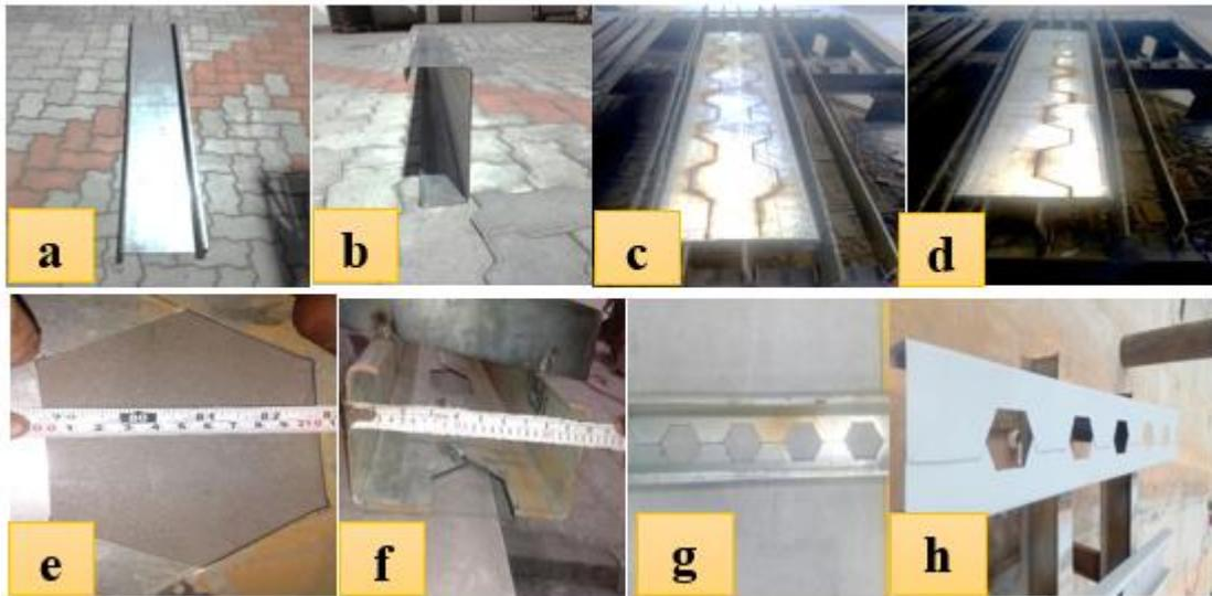
**Fig. 1 - (a) C shaped - Cold formed steel section; (b) cross sectional view- C shaped - Cold formed steel section; (c) plasma torch cutting pattern -1; (d) plasma torch cutting pattern -2; (e) hexagonal dimension pattern verification; (f) overall dimension verification; (g) castellated beam - assembled section; (h) primer coated with finished cold formed metal surface**
