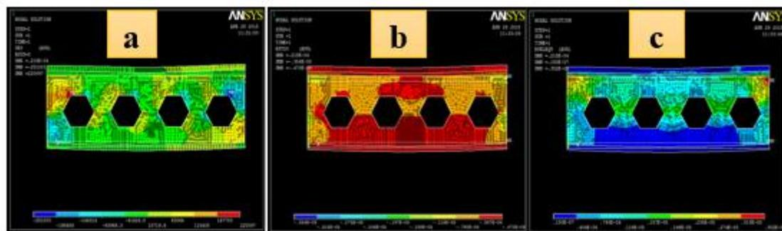
Fig. 8 - (a) XY shear stress contour plot; (b) third principal total mechanical strain; (c) von-mises elastic strain
