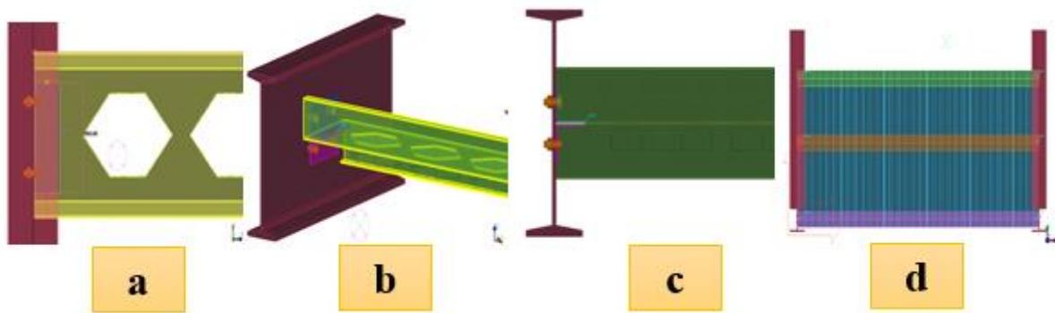
Fig. 3 - (a) Secondary beam column connection detailing in three dimensional view 1 to 3 was marked as a,b,c; (d) decking profile model + Secondary beam connection details
