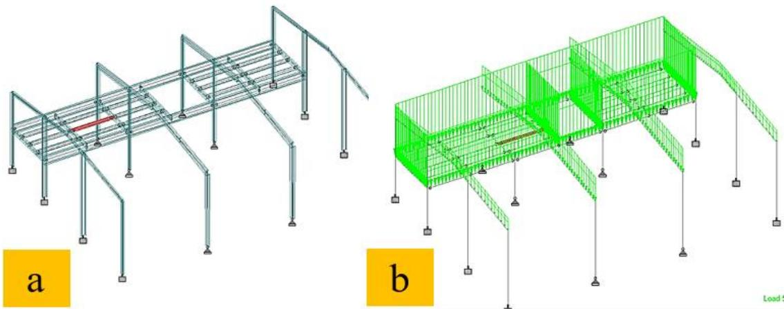
**Fig. 4 - (a) Dimensions & Geometric properties of a Cold formed steel sections; (b) graphical output representation of cold formed steel section**
