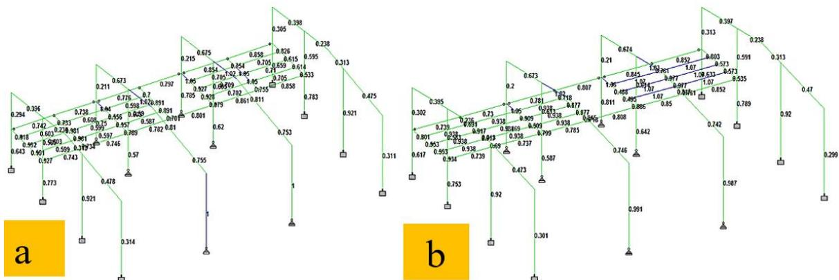
Fig. 7 - Interaction value of; (a) hot steel; (b) CFS steel sections
