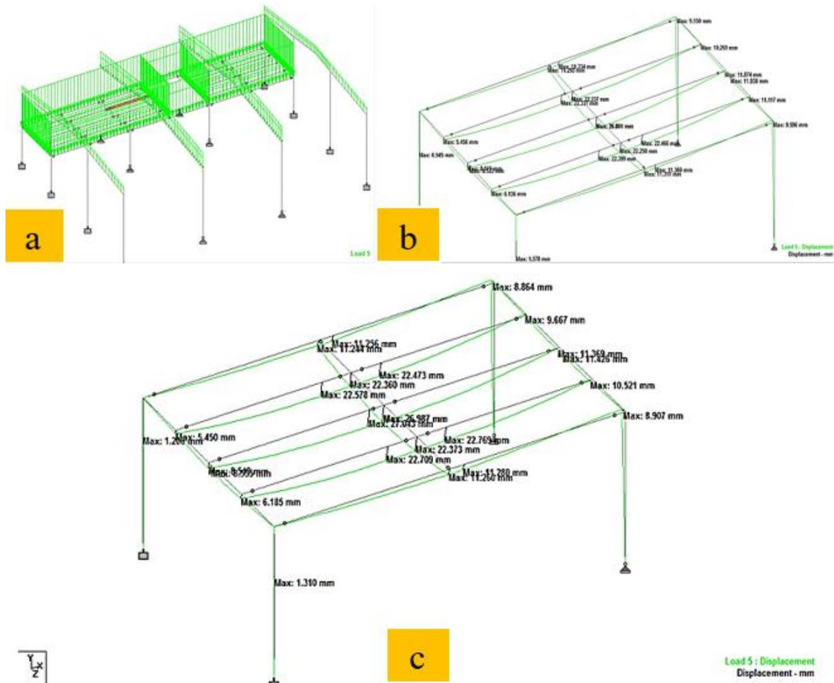
Fig. 5 - (a) Graphical output representation of Hot rolled steel section; (b) deflection value of CFS steel; (c) deflection value in hot rolled steel sections
