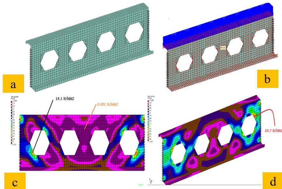
**Fig. 8 - (a) Surface modelling & support condition in STAAD; (b) pressure load applied on the section top flange; (c) stress indication – max absolute case; (d) stress indication – max von-misses formulation**
