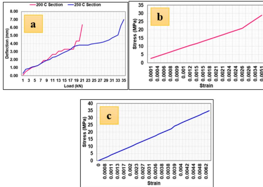
Fig. 6- (a) Deflection vs load curves for 200 C Section and 250 C Section; (b) stress vs strain curve for 200 C Section; (c) stress vs strain curve for 250 C Section
