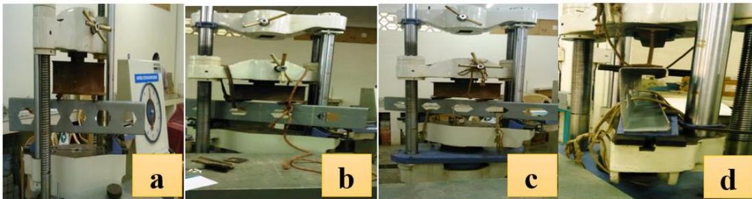
**Fig. 2 - (a) Specimen setting up on instrument; (b) setting up deflection meter; (c) setting out specimen 2 – 250 mm depth; (d) local buckling case under worst loading stage**
