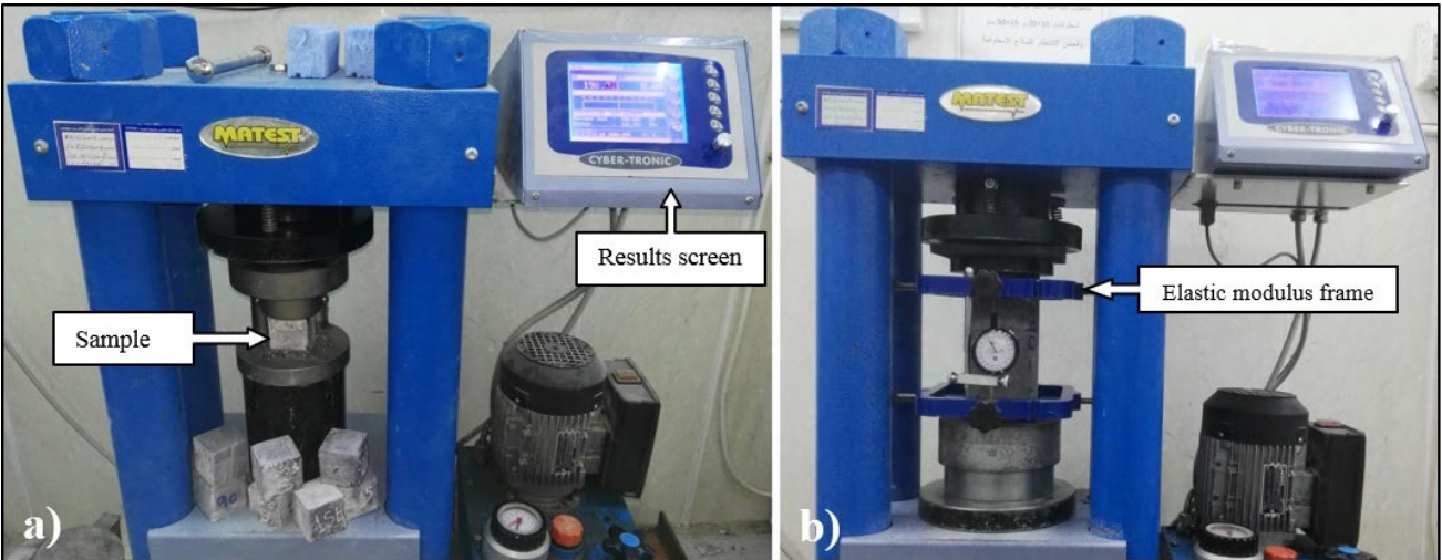
Fig. 4 - (a) Compression test; (b) Static elastic modulus test
