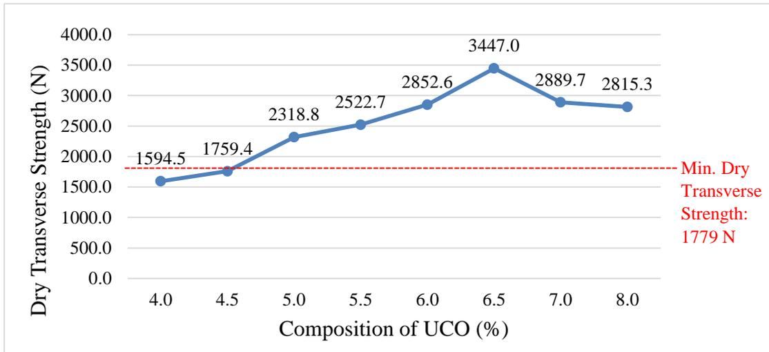
Fig. 4 - Average dry transverse strength and flexural strength achieved by UCO-GRT produced with different composition of binder and filler content
