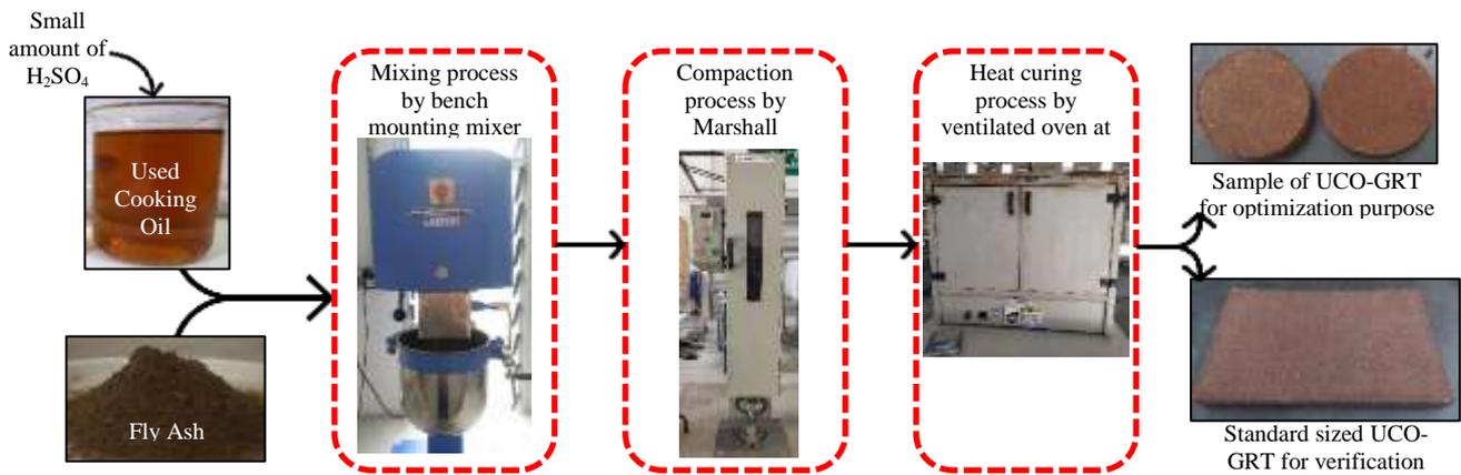
Fig. 2 - Manufacturing process of UCO-GRT
