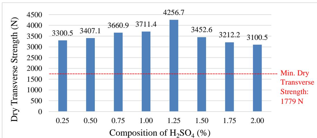
Fig. 5 - The dry transverse strength of UCO-GRT incorporated with different composition of  $H_2SO_4$
