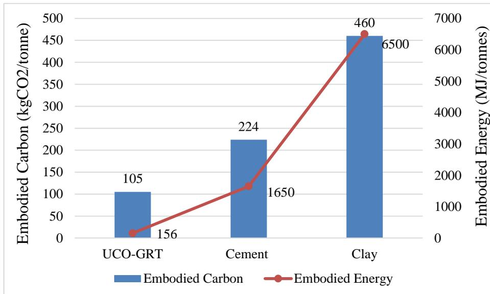
**Fig. 6 - Comparison of the embodied carbon and embodied energy of UCO-GRT, concrete and clay roofing tiles.**
