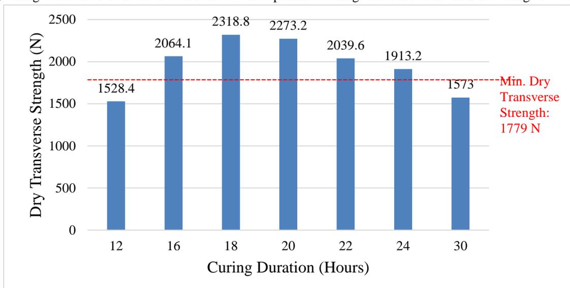
**Fig. 3 - Dry transverse strength of UCO-GRT produced from different durations**
