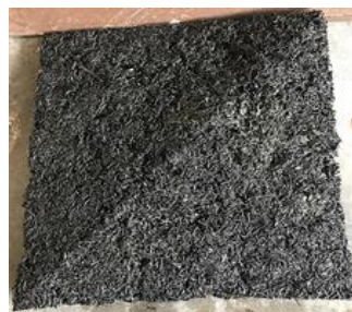
Fig. 4 - Waste Rubber Wall Panel (WRWP)
