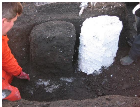
Figure 1. Sampling of in-situ specimens of bottom ash using mesh and gypsum.
