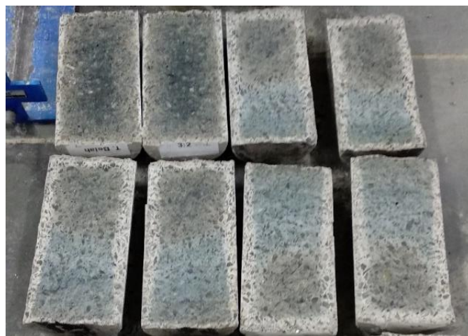
Fig. 8 - Concrete split tensile test
