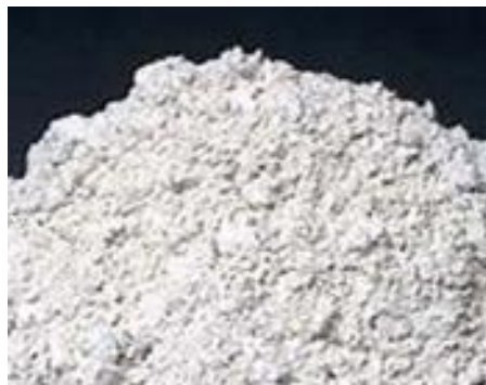
Fig. 3 - GGBFS (Ground Granulated Blast Furnace Slag)
