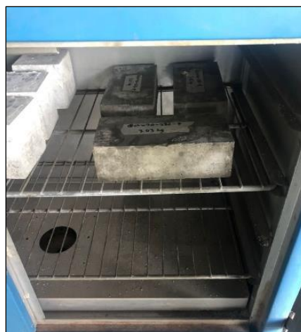
Fig. 6 - The bricks were placed in oven to measure the oven-dry weight
