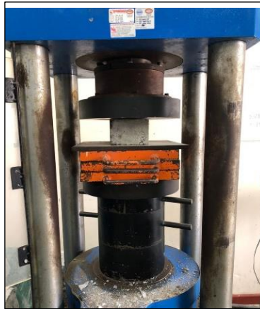
Fig. 5 - Compressive strength testing of brick
