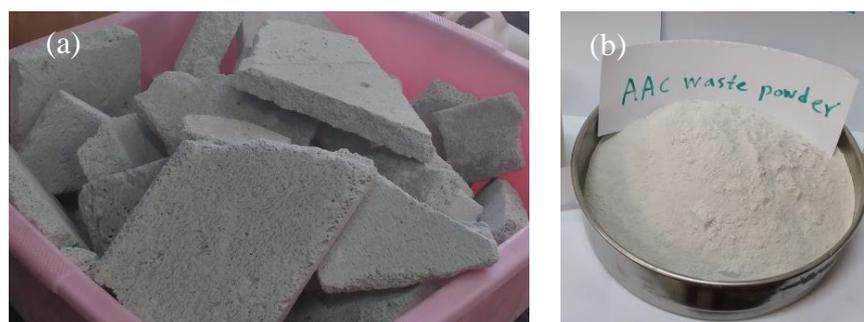
**Fig. 1 - AAC block wastes used in this study; (a) AAC pieces; (b) AAC powder**
