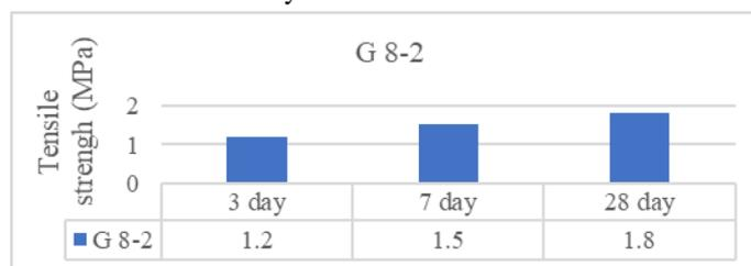
Fig. 10 - Tensile strength of geopolymer mortar prepared from AAC powder passing the sieve No.50 at 3, 7, and 28 days (curing at 80°C)
