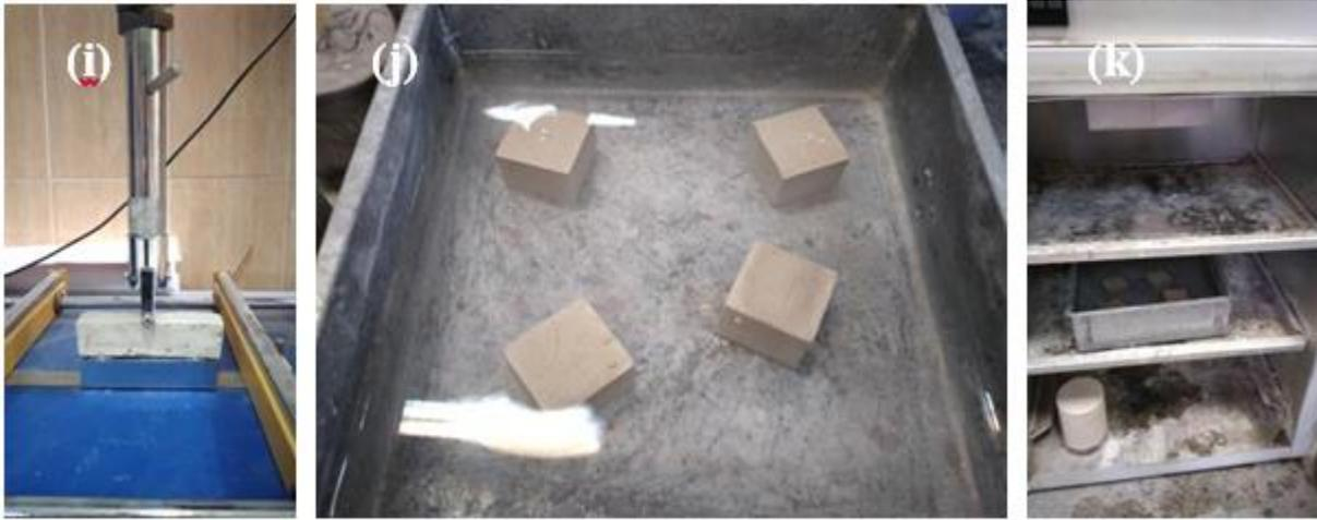
**Fig. 2- Experimental procedure steps; (a) AAC crushing; (b) AAC powder sieving; (c) alkaline solution preparing; (d) mixing the solution with AAC powder; (e) casting; (f) oven-curing; (g) compressive testing; (h) briquette testing; (i) flexural testing; (j) immersion water absorption testing; (k) boiling water absorption testing**
