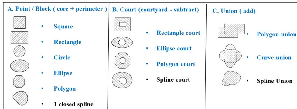
**Fig 7 - 13 Types of massing shapes in three major categories 10 regular shapes and 3 splines free-form generated for the sample site**
