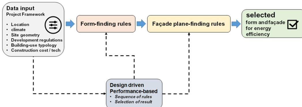
Fig. 3 - The overall process of form-finding and façade plane finding
