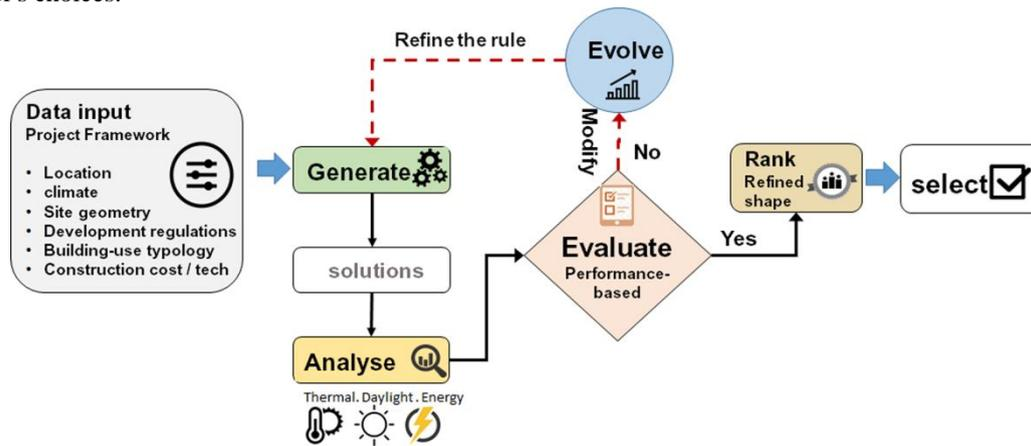
Fig. 2 - Overall process of PBSG rule for the generative design
