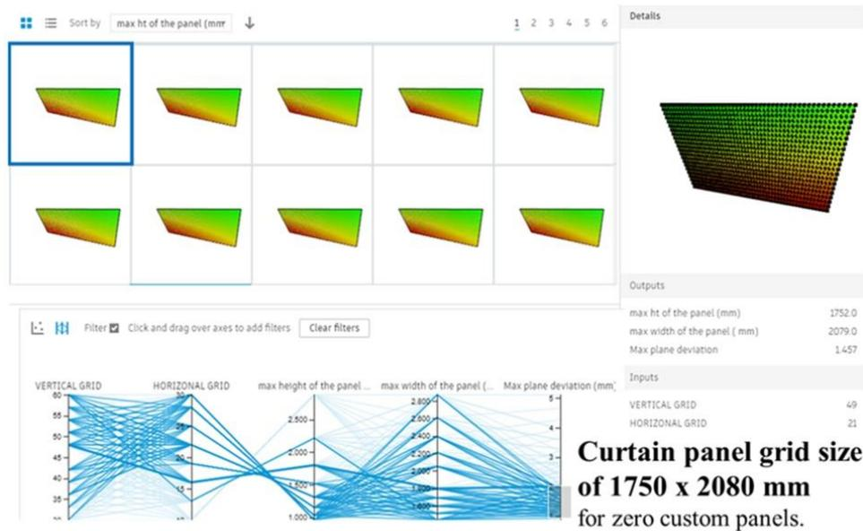
**Fig. 18 - Rule 5, plane deviation and maximum panel size for < 2mm deviation in the south glazing façade plane**
