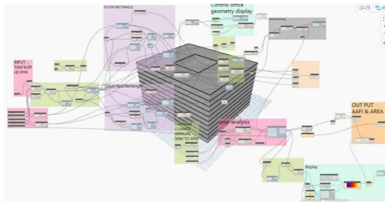
Fig. 12 - Dynamo geometry script for output results for solar insolation and façade area in the rectangular court form typology
