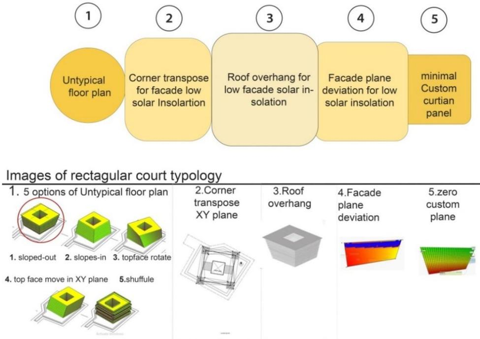
Fig. 14 - Shape grammar process and rules for façade plane- finding
