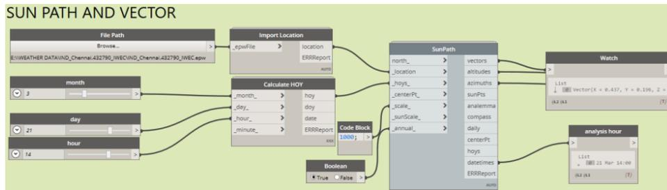
Fig 8 - Sun path node from Ladybug for Dynamo
