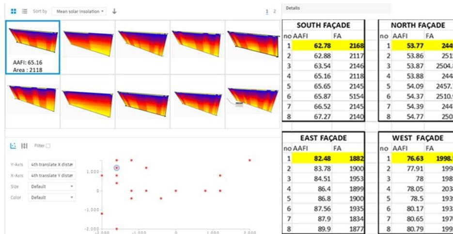
Fig 17 - Rule 4, solar insolation by façade corner transpose in project refinery and the data chart for all the planes
