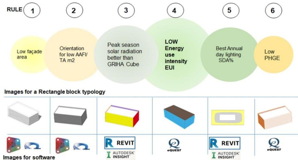
Fig. 11 - Six shape grammar rules process for form finding with case sample rectangle form generative process and software used
