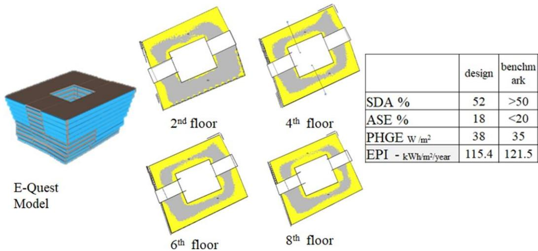
Fig. 19 - SG finalized form final results energy model, SDA floor plans and table of results
