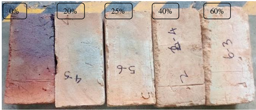
Fig. 7 - Burnt bricks with different fly ash contents
