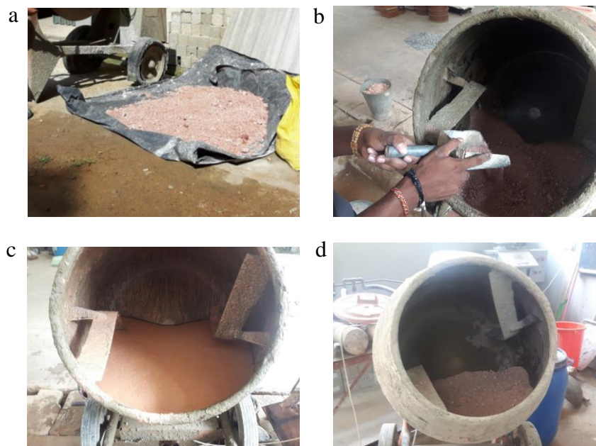
Fig. 1 - (a): Dry soil; (b) put in the concrete mixer; (c) mix with water; (d) clay slurry after washing
