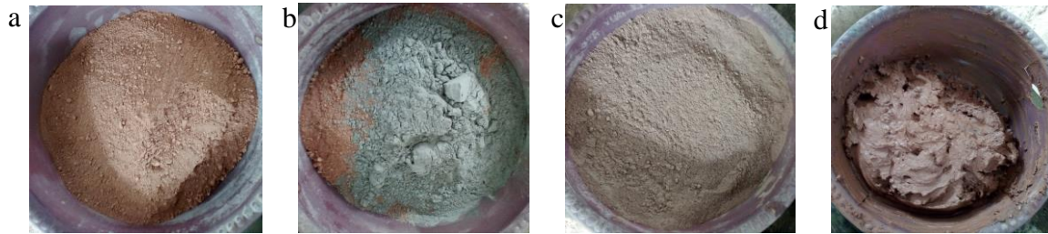
Fig. 3 - Preparation of clay mix for burnt bricks production (a) extracted clay; (b) add fly ash; (c) mix of clay and fly ash; (d) mix with water
