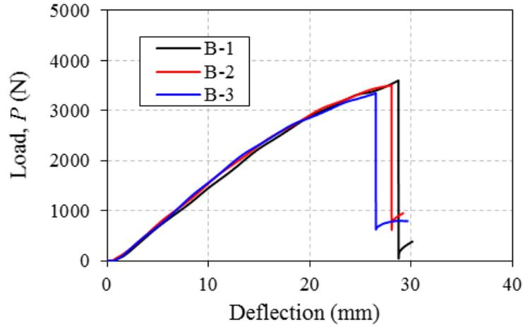
Fig. 6 - Load-deflection behavior for CFS plate strengthened beams (type B)
