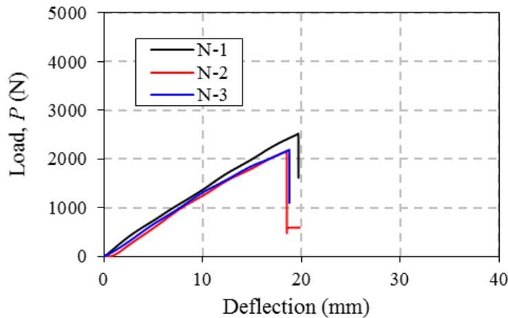
Fig. 4 - Load-deflection behavior for control unstrengthened beams (type N)
