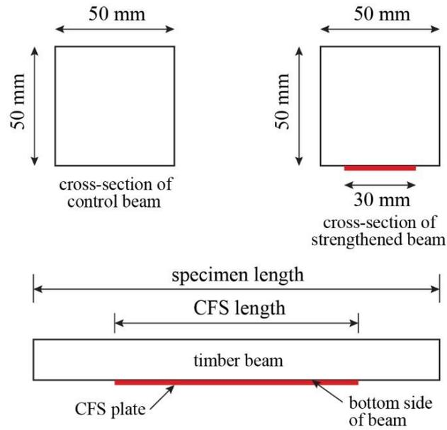
**Fig. 1 - Dimension and configuration of test specimen**
