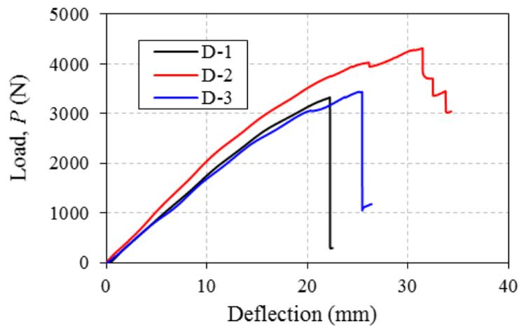
Fig. 8 - Load-deflection behavior for CFS plate strengthened beams (type D)
