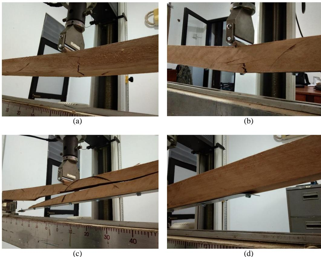
**Fig. 9 - Failure modes of tested beams (a) brittle failure in control beams; (b) tensile-flexural failure in strengthened beams; (c) shear failure in strengthened beam; (d) screw pulled out at the end of CFS plate**
