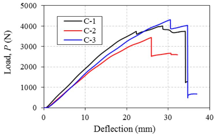
Fig. 7 - Load-deflection behavior for CFS plate strengthened beams (type C)
