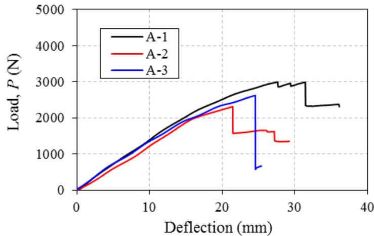
Fig. 5 - Load-deflection behavior for CFS plate strengthened beams (type A)
