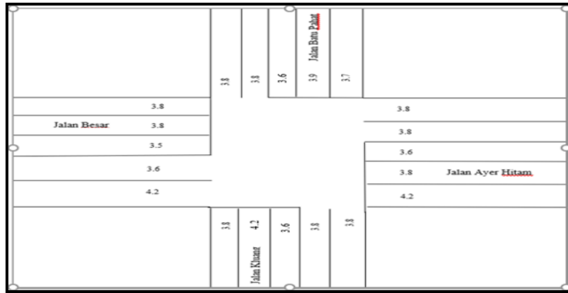
Fig. 3 - Geometry at Ayer Hitam signalised intersection
