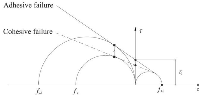
**Fig. 3 - Failure envelope using Mohr-Coulomb theory**
