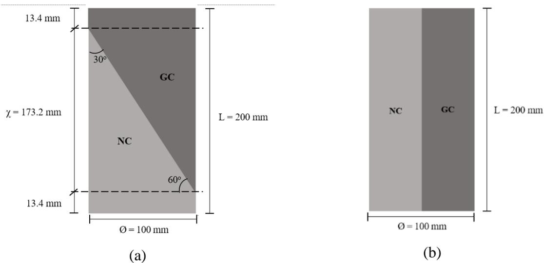
Fig. 1 - Dimension of bond substrate
