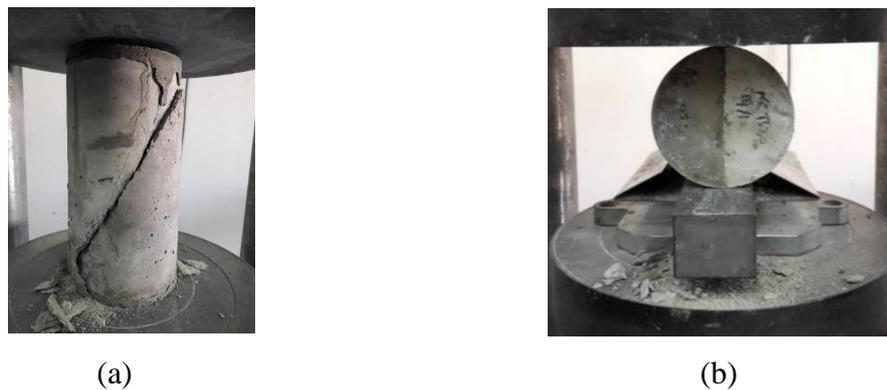
Fig. 2 - Bonding test (a) slant shear test and; (b) split tensile
