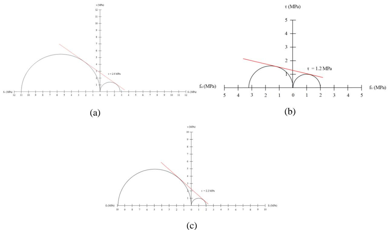
**Fig. 4 - Adhesive bond failure envelope using Mohr-Coulomb theory (a) NC30-GC80; (b) NC30-GC85 and; (c) NC30-GC90**
