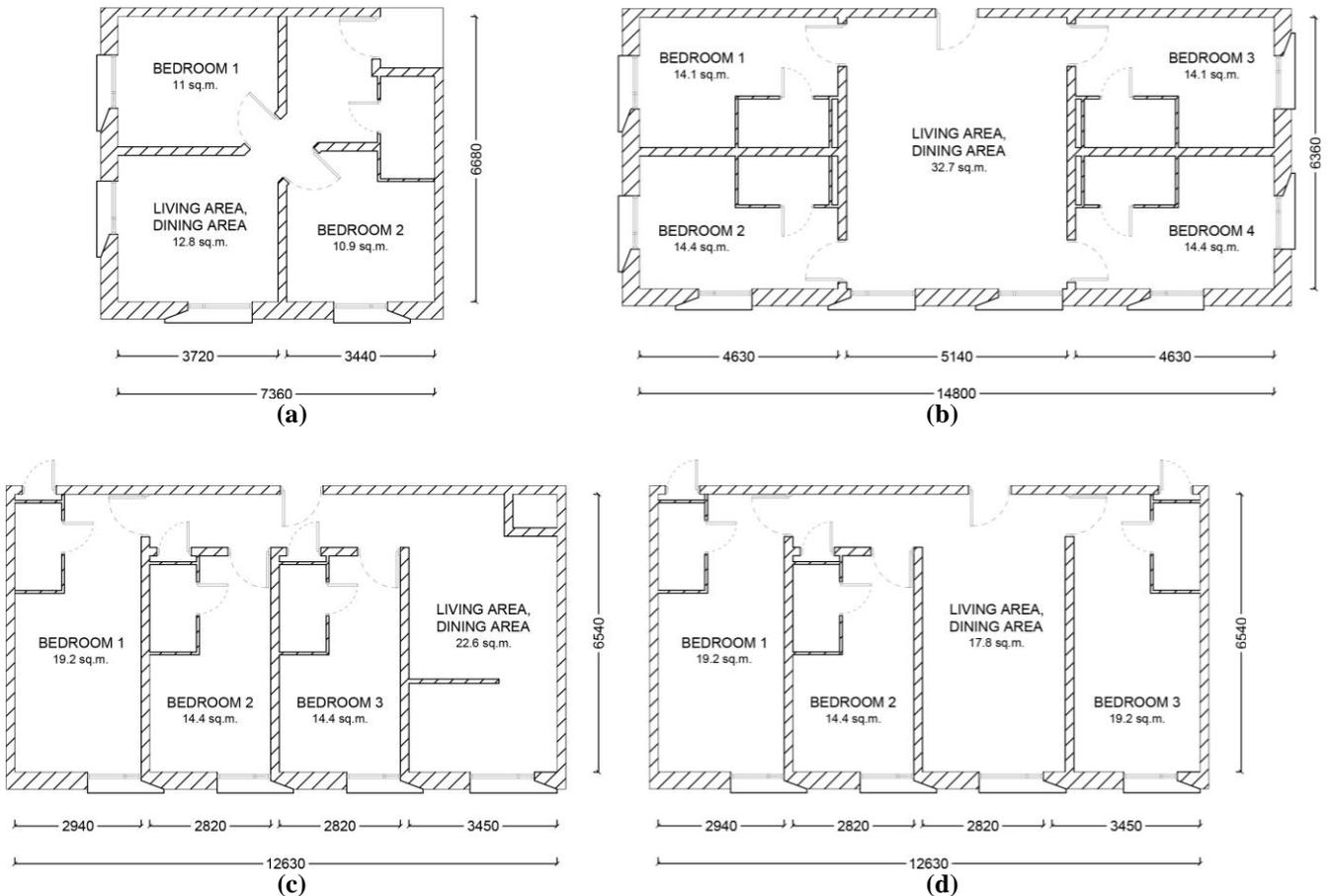
Fig. 6 - Floor plan of the co-living units (source: Manchester City Council, 2018) (a) twodio type; (b) 4-bed type; (c) 3-bed type 1; (d) 3-bed type 2
