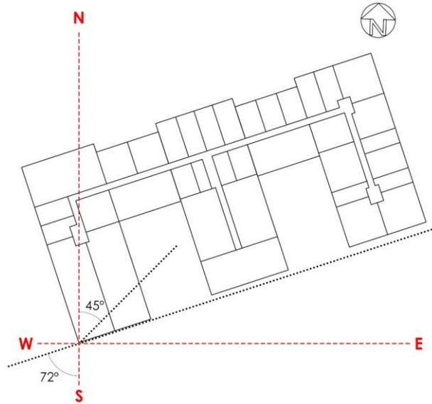
**Fig. 7 - Building orientation: main façade facing within 90° due South and avoiding 45° due North as suggested in the BRE Guide (source: Author’s diagram)**
