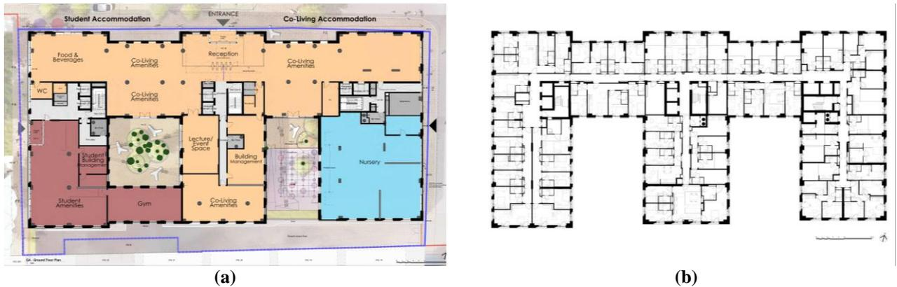
Fig. 4 - (a) Ground floor plan of the Echo Street Co-Living. The drawing is not to scale (source: Manchester City Council, 2018); (b) typical floor plan (source: Manchester City Council, 2018)
