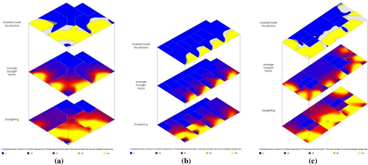
**Fig. 9 - Sefaira Visualization on the co-living units (a) twodio unit; (b) three-bed unit; (c) four-bed unit**
