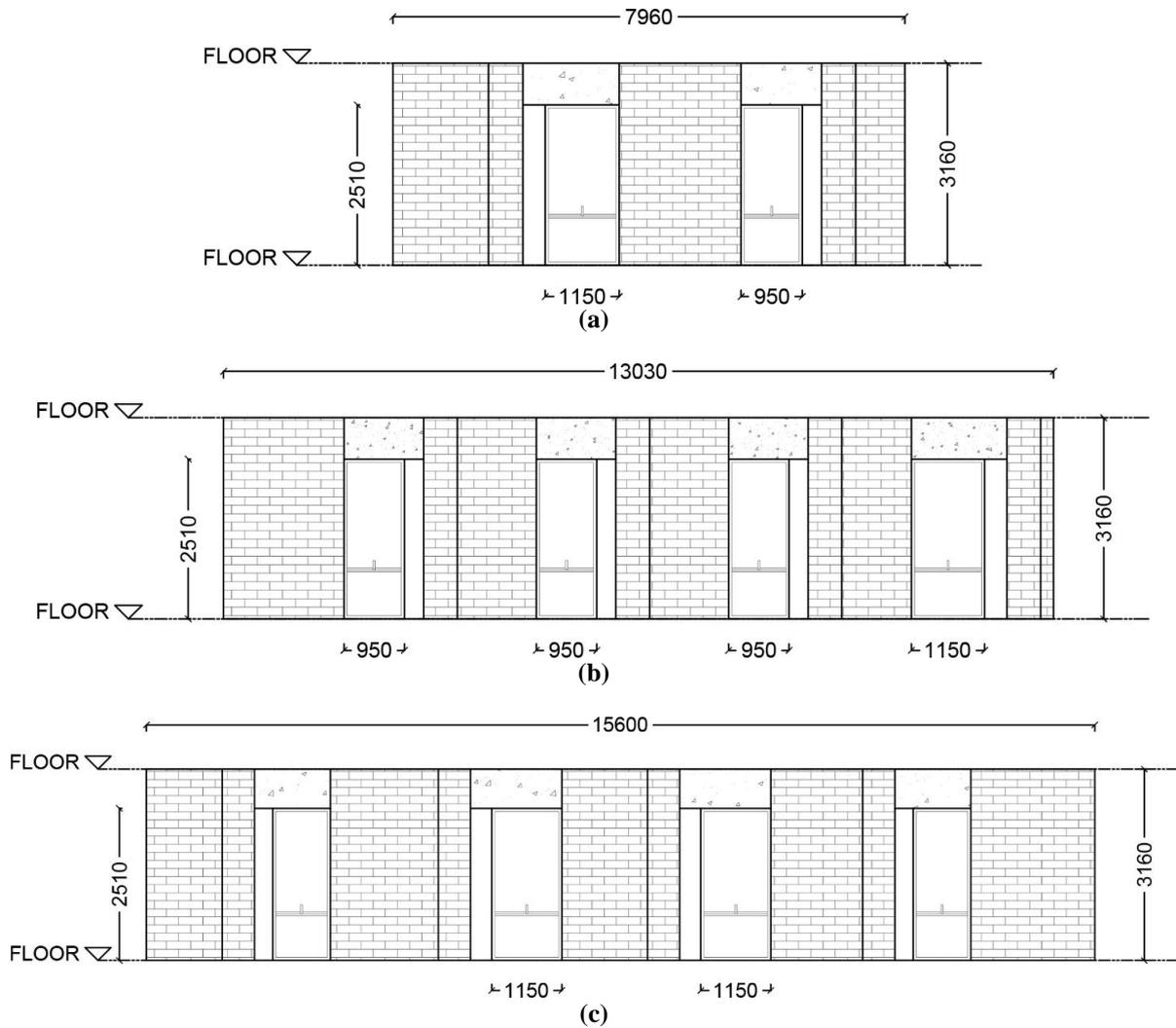
**Fig. 8 - Co-living units elevation view (source: Manchester City Council, 2018) (a) twodio unit; (b) three-bed unit; (c) four-bed unit**
