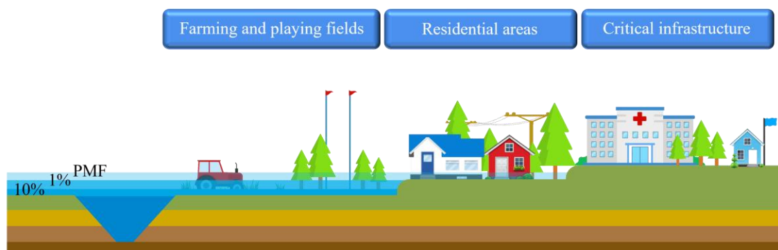
Fig. 9 - Critical public infrastructure such as hospitals and emergency management centres are ideally located outside the influence of Probable Maximum Flood (PMF). Note that a 10% flood is 1 in 10-year flood and 1% flood is a 1 in 100-year flood (Queensland Government, 2011)
