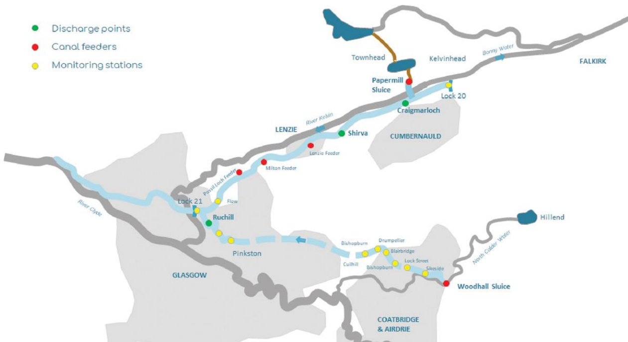
Fig. 6 - Schematic of Glasgow’s Smart Canal infrastructure. During normal operation, default positions of discharge sluices are closed and feeder sluices are open (Hay-Smith, 2022)
