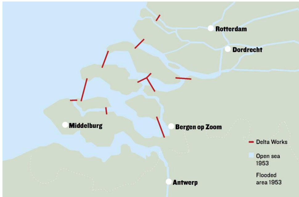
Fig. 1 - Delta Works consisted of storm surge barriers, dams, sluices and dykes close off streams of delta from the sea and keep the land safe from floods (Rietveld et al., 2017; Pilarczyk, 2006)
