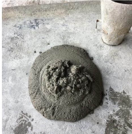
Fig. 2 - Spread of foamed concrete
