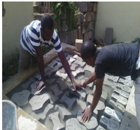
(c) Curing of paving stones
