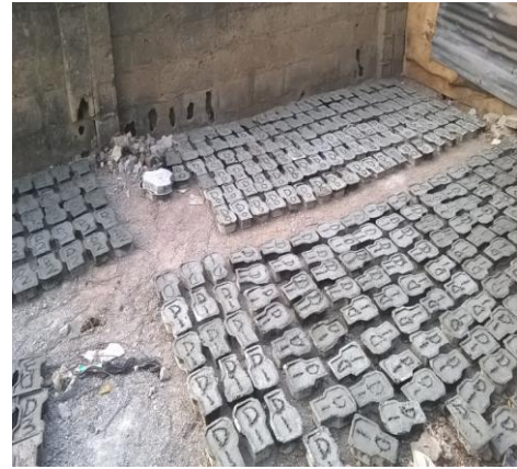
(b) Produced paving stones
