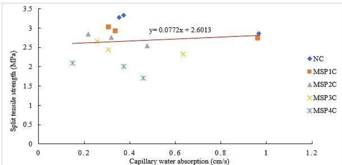
Fig. 10 - Relationship between split tensile strength and capillary water absorption on 7, 28 and 90 days curing
