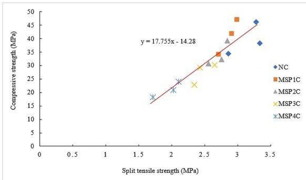
**Fig. 8 - Relationship between compressive strength and split tensile strength on 7, 28 and 90 days curing**
