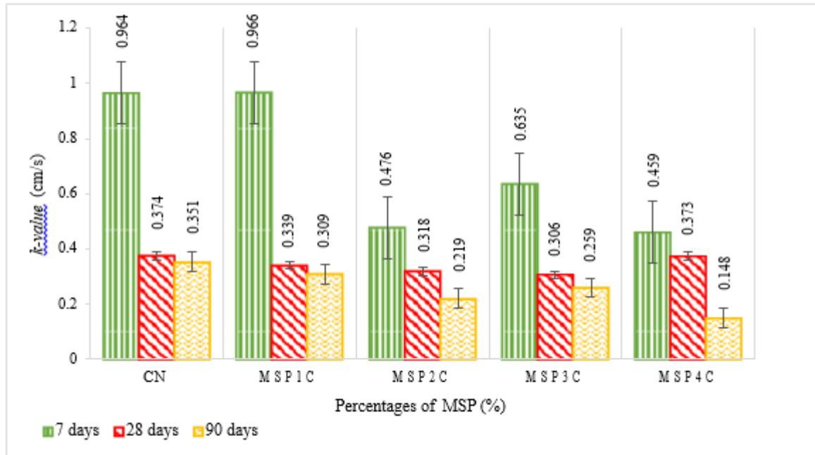
Fig. 7 - Capillary water absorption of concrete
