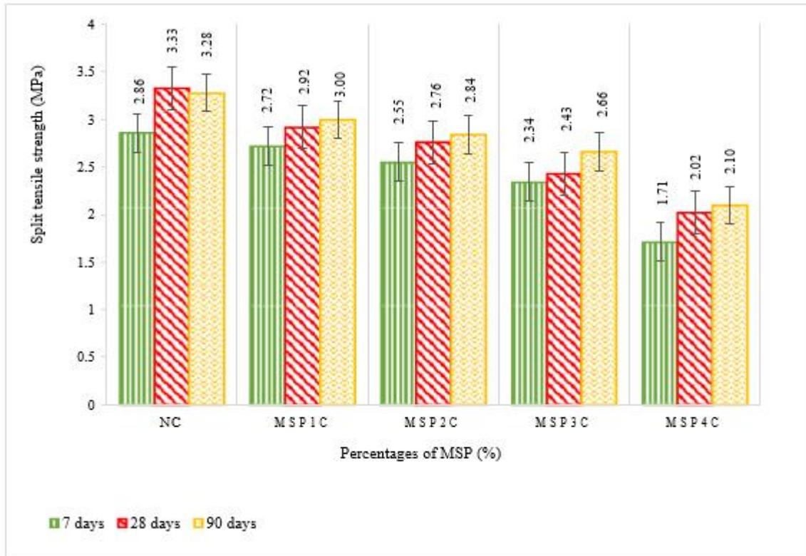
Fig. 6 - Split tensile strength concrete specimens
