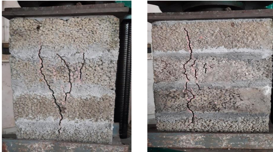
Fig. 12 - (a) QB00 Prism failure pattern (b) QB03 Prism failure pattern
