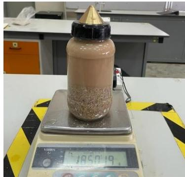
**Fig. 4 - Specific gravity test of sand and construction tiles waste (CTW)**
