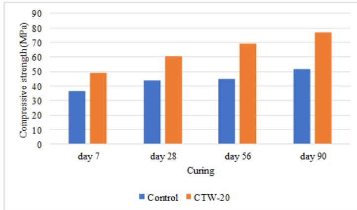
**Fig. 7 - Compressive strength of control and CTW-20**
