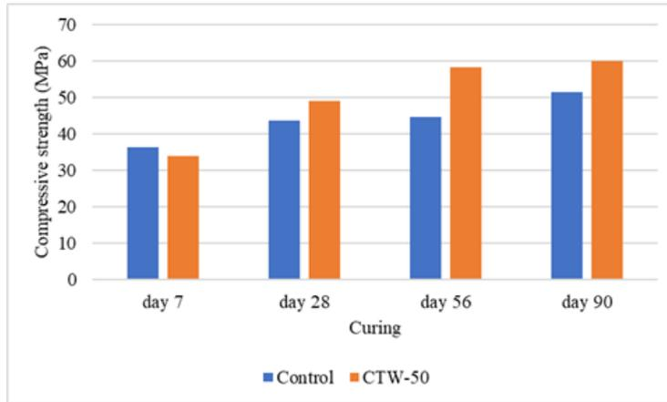
Fig. 10 - Compressive strength of control and CTW-50
