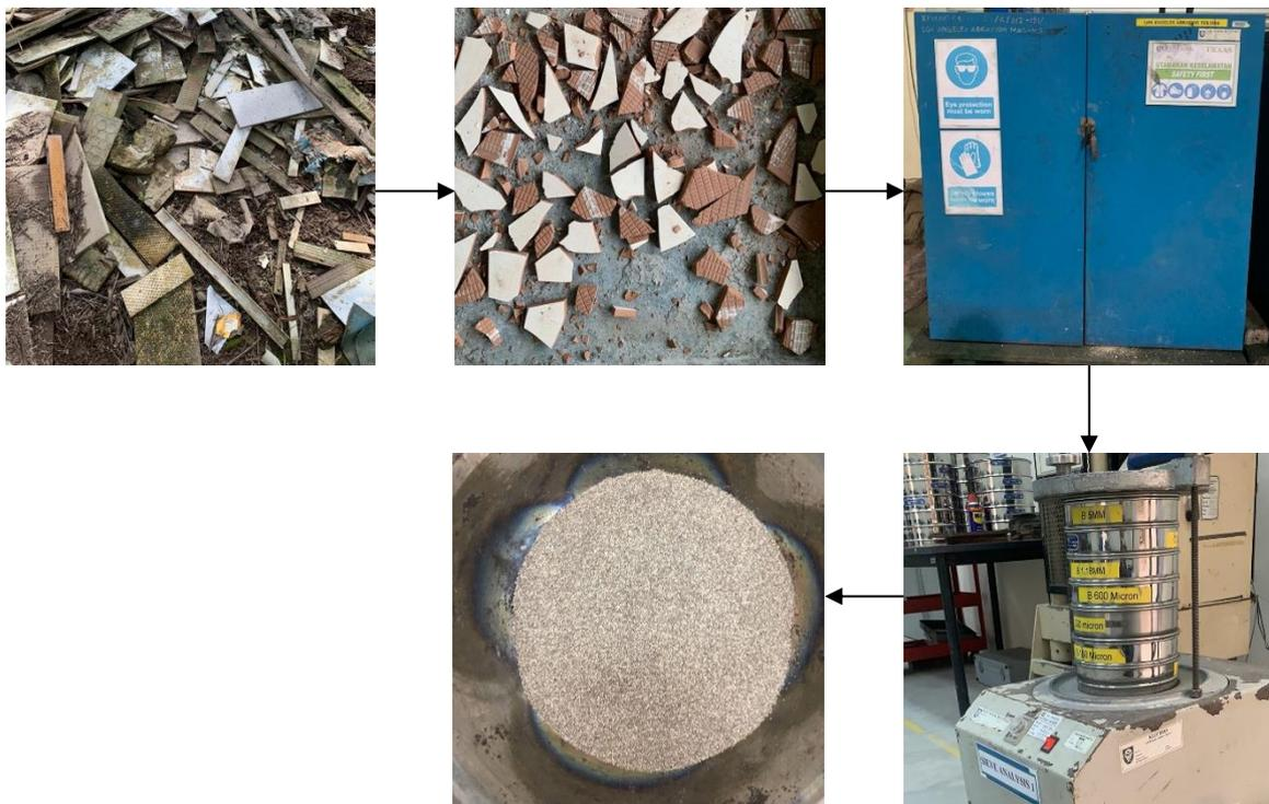
Fig. 2 - Process of grinding construction tiles waste (CTW)
