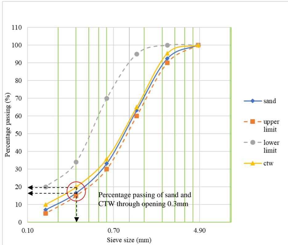
**Fig. 3 - Sieve analysis result of sand and construction tiles waste (CTW)**
