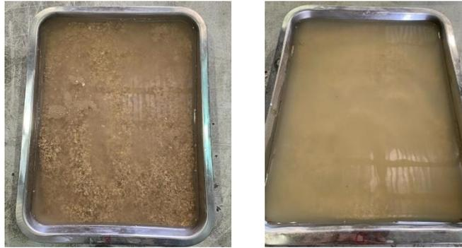
**Fig. 5 - Water absorption test of sand and construction tiles waste (CTW)**
