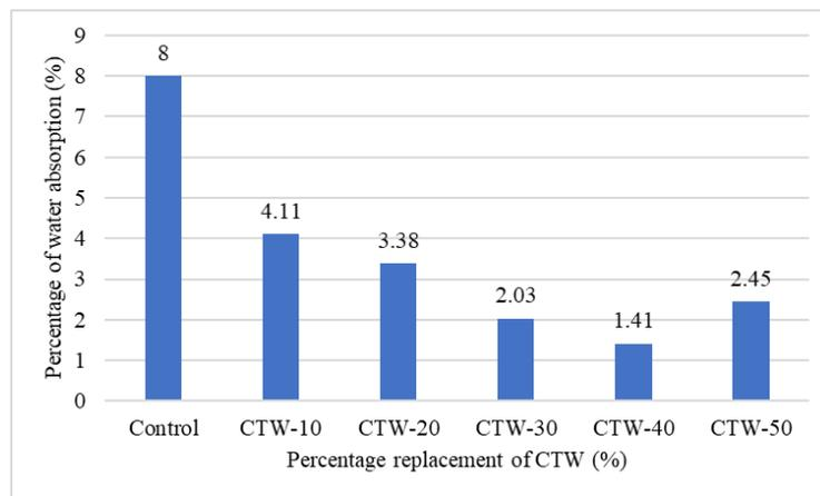
**Fig. 13 - Percentage water absorption of control at 56 days of curing**
