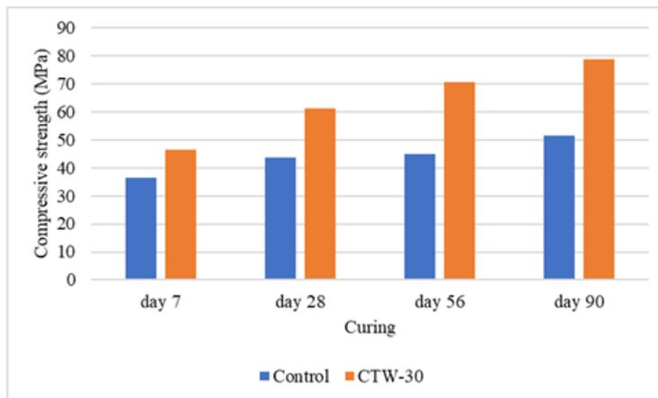
**Fig. 8 - Compressive strength of control and CTW-30**
