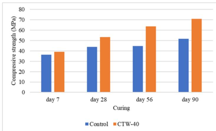
**Fig. 9 - Compressive strength of control and CTW-40**
