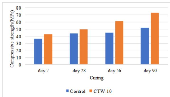
**Fig. 6 - Compressive strength of control and CTW-10**
