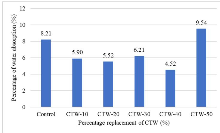
**Fig. 12 - Percentage water absorption of control at 28 days of curing**
