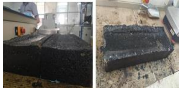
Fig. 11 E3 mixture before and after rutting
