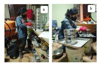
Fig. 2 (a) Granulometry performed for fine aggregates, (b) granulometry performed for coarse aggregates
