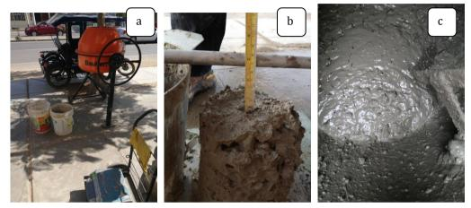
Fig. 4 (a) Elements used for concrete preparation, (b) Slump measurement, (c) Concrete mixed with fiber additions
