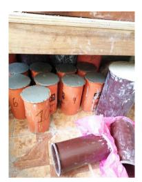
Fig. 7 Filling of test specimens for testing NTP 339.084
