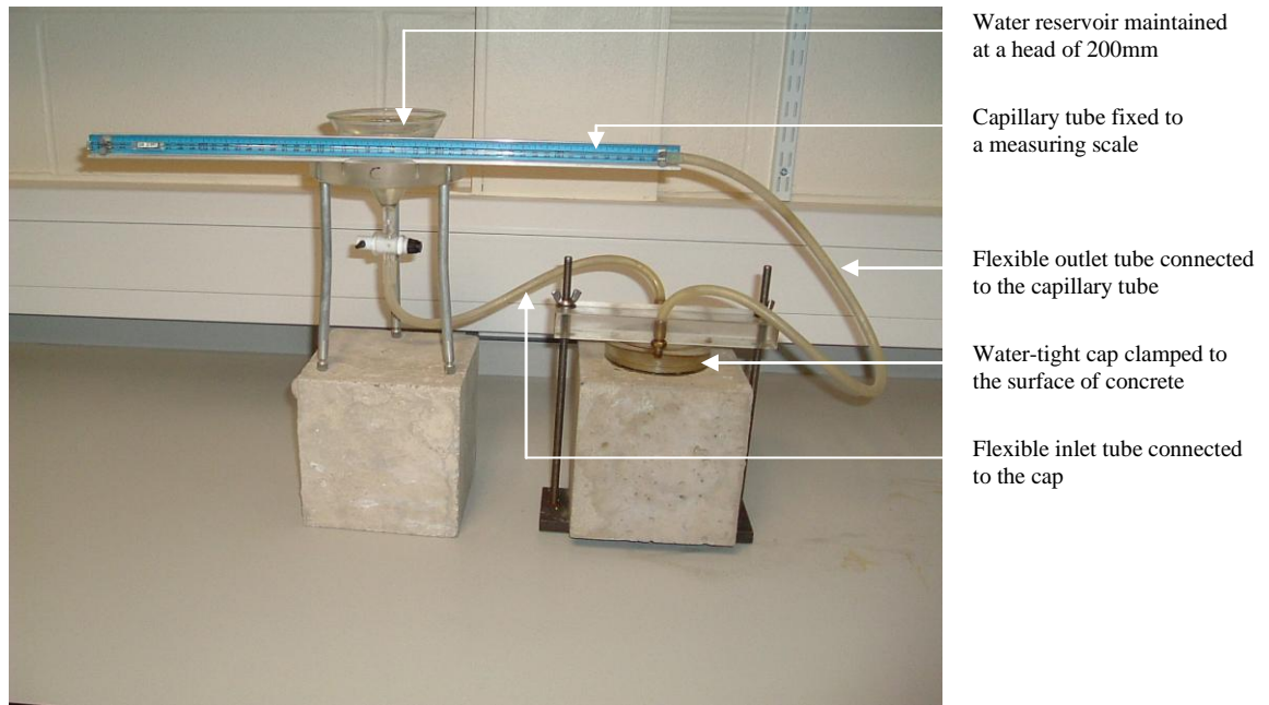
Figure 1: A typical ISAT set-up
