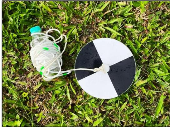
Fig. 2 - Secchi Disc are used to measure water transparency
