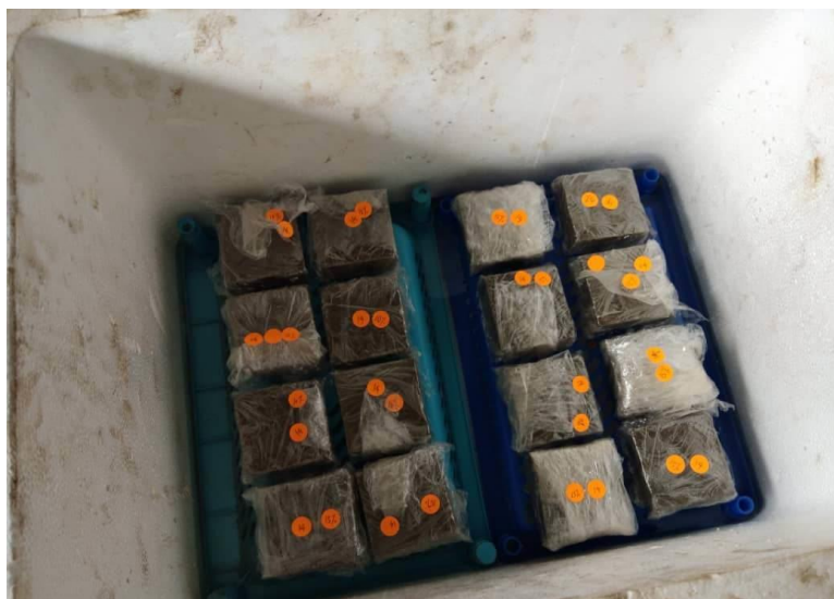
Fig. 3 Specimens preparation for direct shear test
